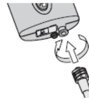
Check tube connection
